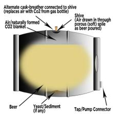
allowed to settle in the cellar! As the beer is drawn out, air is drawn in either through a porous spile placed in the shive or, if the cask is vertical, through a breather tube at the top. There is a device called a 'cask breather' that feeds carbon dioxide (CO<sup>2</sup>) at low pressure to replace the beer drawn out. This is instead of letting the cask breathe through the spile/breather but does not pressurise the cask at all. Some drinkers don't approve but they are now recognised by CAMRA.
